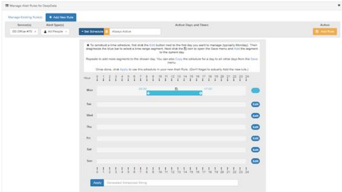
Monday would already have the edit mode open. You can now set the time you would like to be alerted for, with the blue bar, by dragging it to the time slot required. You can shorten and/or lengthen the bar as well, by clicking on the left arrow, on the right hand side within the bar.
